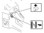
If the machine is fitted with an air purge (A): Press the air purge repeatedly until fuel begins to fill the bulb. The bulb need not be completely filled.
